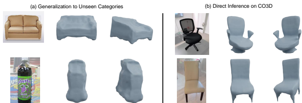
Figure 9. (a) Reconstruction on unseen categories. (b) Inference of our Pix3D-trained model on CO3D chairs.
